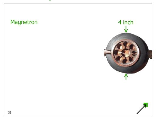
But there was a big problem. The heart of the radar, the magnetron transmitter tube, required a complex shape machined into a internal solid block of copper. A skilled machinist labored two weeks to make one.
